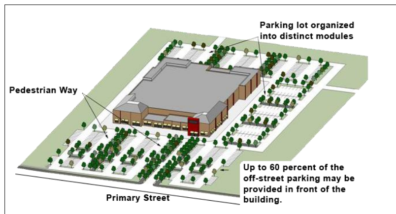
Figure 5.7.F(5): Large Retail Parking Lot with Over 200 Spaces
