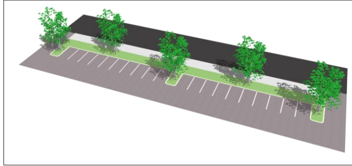
Figure 5.3.H(5)a.1(b): Interior Parking Area Minimum Plantings
